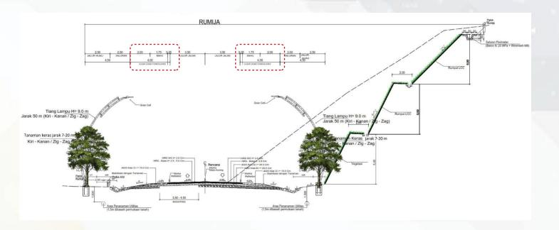
Typical Cross Section on Labuan Bajo –SP. Nalis – SP. Kenari - Tanamori Road used 3,5 m traffic lane with 4 m Clear Zone (2 m shoulder and 2 m foreslope)
